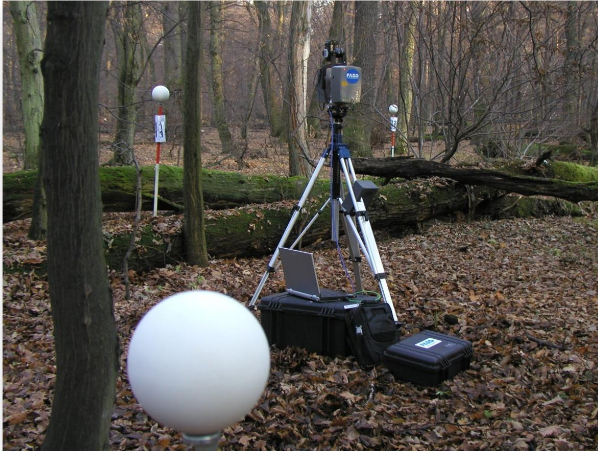
TLS 2006 Scanner Faro LS 880
